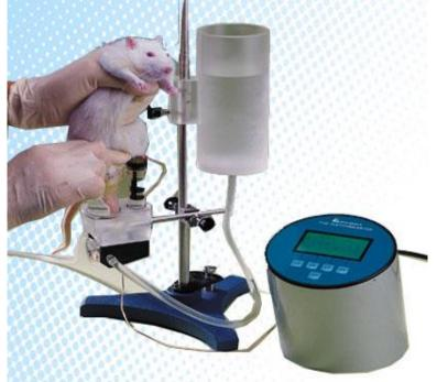
The Ugo Basile<sup>™</sup> **Plethysmometer** is a microprocessor-controlled volume meter that has long been the standard instrument for measurement of rodent paw volume.
