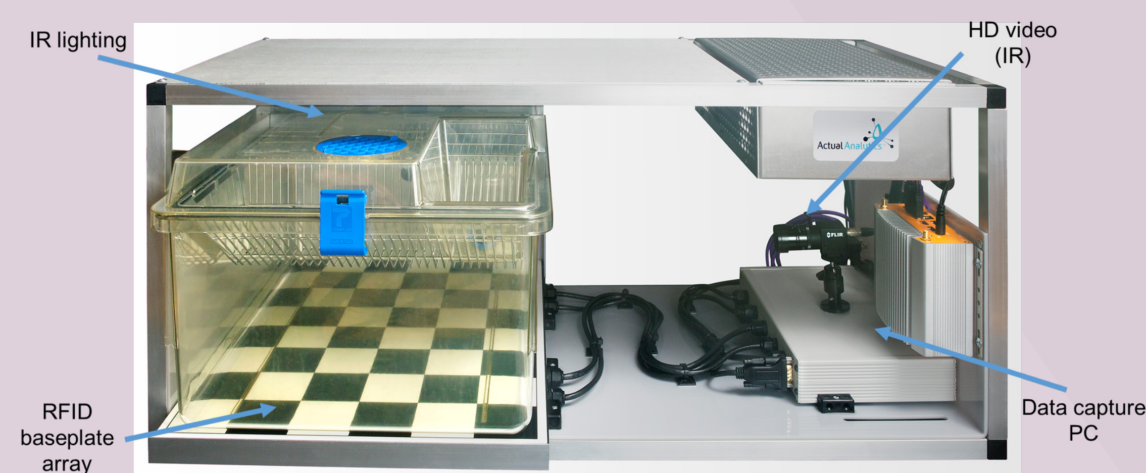
Figure 1. The Home Cage Analyser (ActualHCA™) system. The system is compatible with IVC home caging and for the current study four systems were installed in a Techniplast blue-line rack. An RFID baseplate array sits under the cage with 12 antennae scanning at ~1Hz provides monitoring of location and temperature of each individual tagged animal. This is then used to generate the temperature, locomotor activity and social proximity data. Top mounted infrared lights and a side mounted infrared camera continuously records 25Hz HD video footage for on-demand review of any significant events and permits automated behaviour recognition using computer vision and machine learning algorithms. The system is currently able to identify temperature, a range of ambulatory and vertical activities, eating, drinking, rearing and social interactions.
