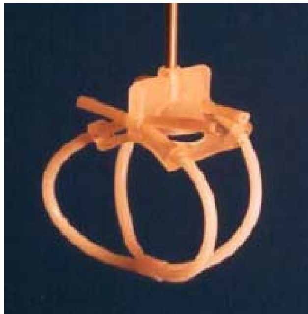
Figure 3. A harness used for rats. Similar harnesses are available for other species.
