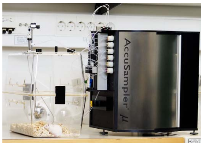
Figure 1. A mouse connected to the AccuSampler® via a catheter. A spring tether is used to protect the catheter and extension line leading up to a swivel, which is mounted on a spring-balanced lever arm.
