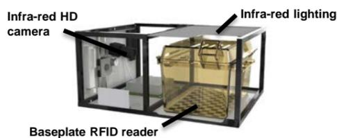
Figure 1: A schematic diagram of an enclosure set up in a conventional cage rack.
